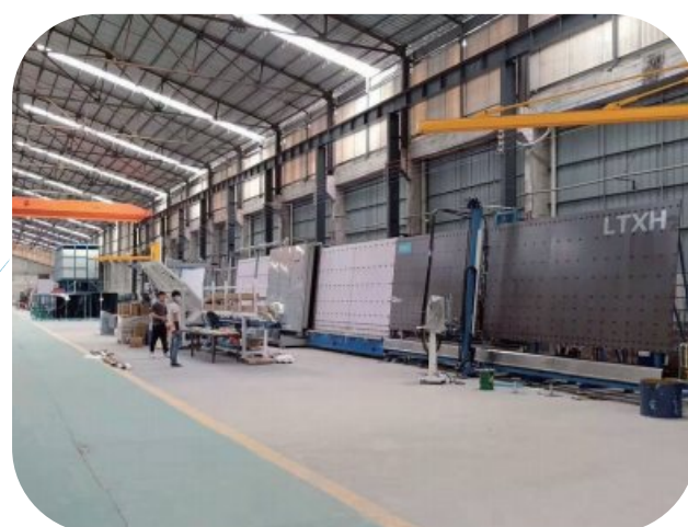
Insulated production line
